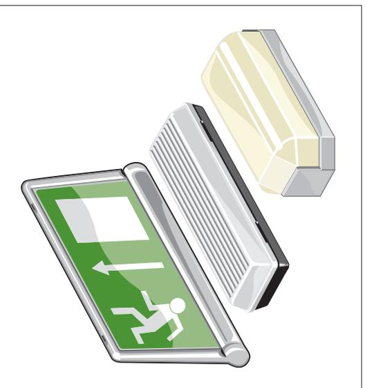
Emergency escape lighting luminaires can be stand-alone dedicated units or incorporated into normal light fittings. There are highly decorative versions of these for those areas that demand aesthetically pleasing fixtures. Power supplies can be rechargeable batteries integral to each unit, a central battery bank or an automatic start generator.
