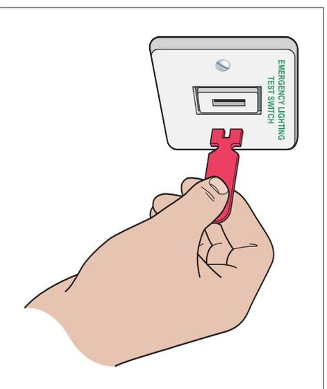
Test facilities often take the form of a 'fish-tail' key (see Figure 50) inserted in a special switch either near the main fuse board or adjacent to relevant light switches.
