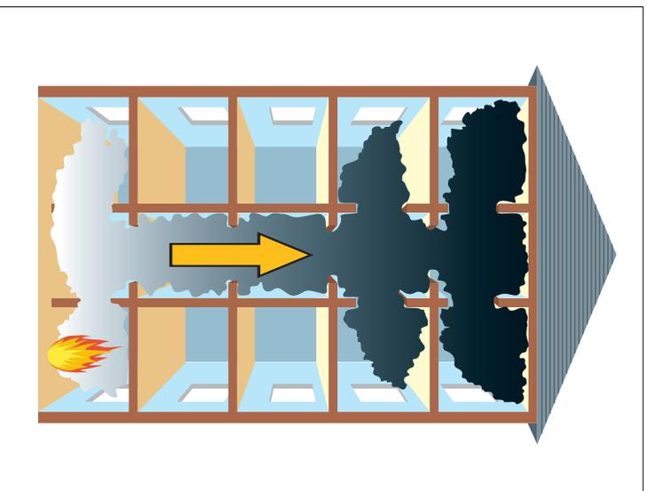
*Figure 5: Smoke moving through a building*
