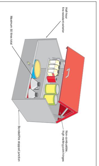
Figure 16: A 50 litre flammable storage bin
