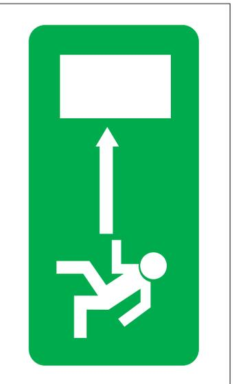
The legibility of escape signs is determined by the size of the sign, its level of illumination and the distance over which it is viewed. The use of signs within the same premises should follow a consistent design pattern or scheme. You should not rely on a few outsized signs which may encourage people to travel to a particular escape route when other more appropriate routes should be used.
